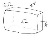
Let *h* be enthalpy ("energy") density in  $\Omega \subset D$ . The rate of change of the total quantity within  $\Omega$  equals the negative of the net flux through  $\partial\Omega$  plus energy sources/sinks:
